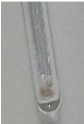
Figure 2: After heating the sample at around its melting point (235 degree celsius), the sample was burnt before melting.
